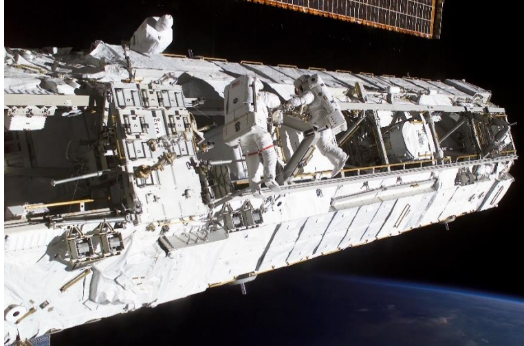
Figure 2 – Picture of ISS Truss Segment and close-ups of frame. Frame is roughly 12” wide with 1/8” thick edges (exact dimensions will be provided).
